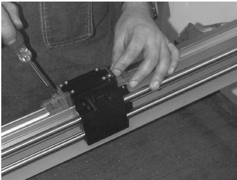
Figure 11-41 Attach Throw Rod Mounting Bracket to Scale Reader
