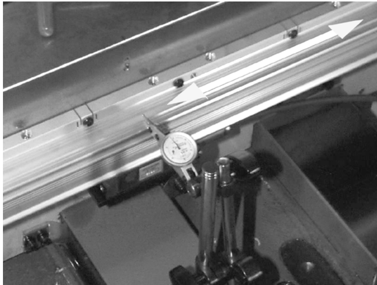
Figure 11-24 Mount Scale to Table
