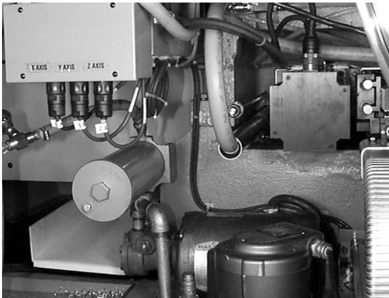
Figure 11-57 Route Cables to Back of Control Cabinet
