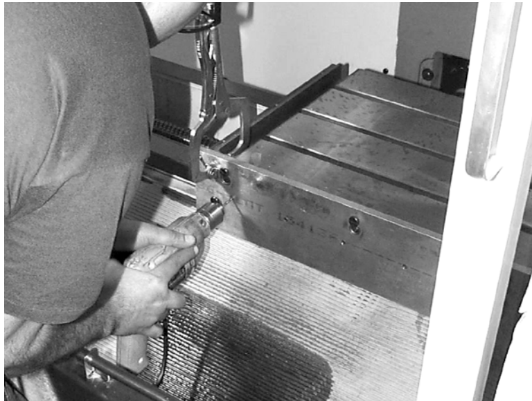
Figure 11-7 Drill Starting Holes
