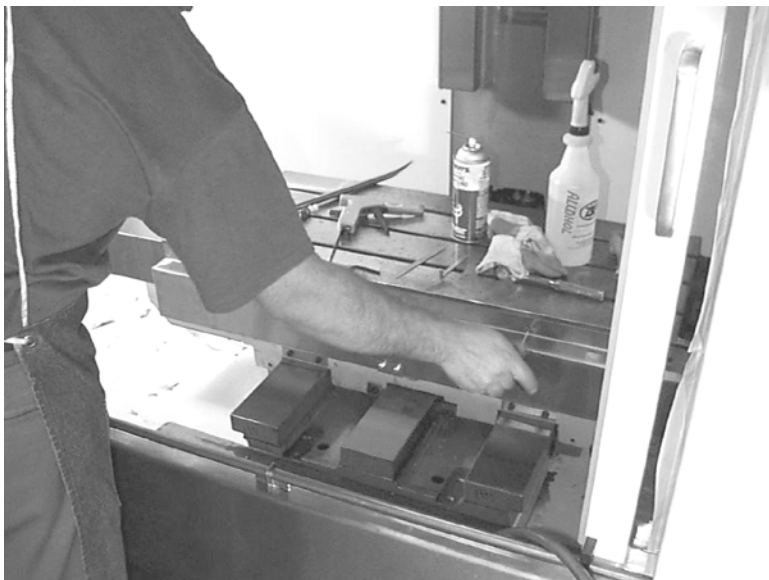
Figure 11-30 Attach Axis Position Indicator to Scale Cover
