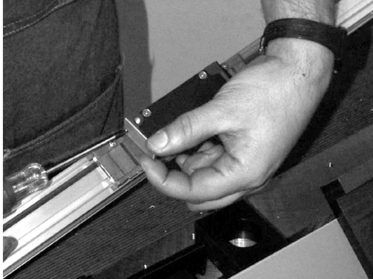
Figure 11-19 Remove Protective Cover from Pin Connector
