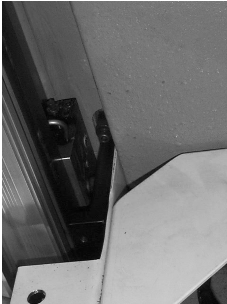
Figure 11-70 Attach Z Axis Mounting Bracket to Column
