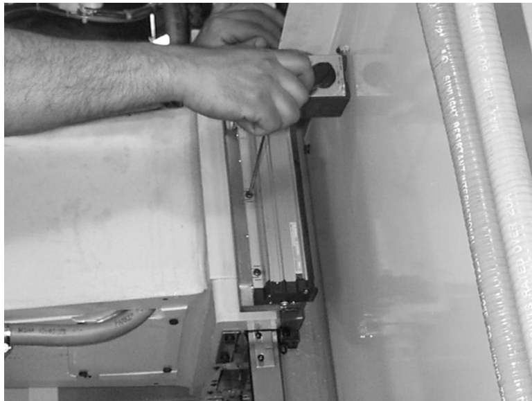
Figure 11-68 Attach Scale to Mounting Plate
