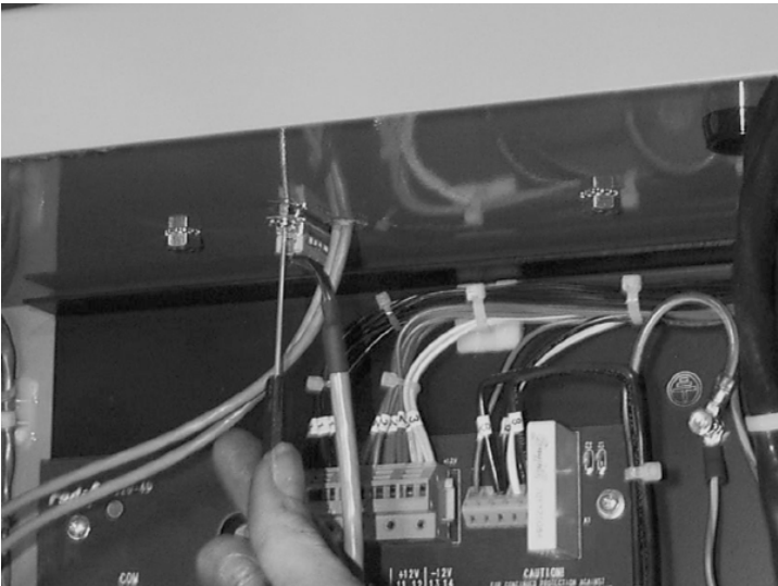
Figure 11-101 Plug 15 Pin Connector into Scale Box Connector
