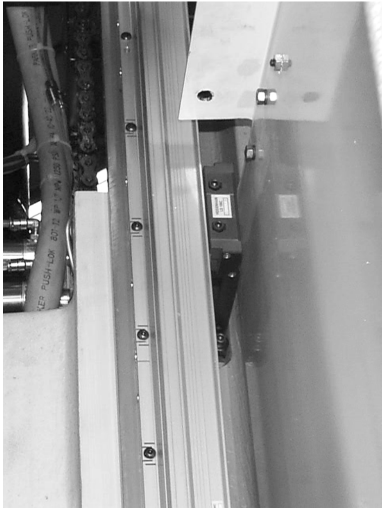
Figure 11-71 Attach Scale Reader to Mounting Bracket
