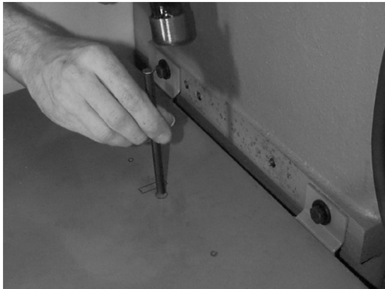
Figure 11-92 Center Punch Hole Locations for Drilling
