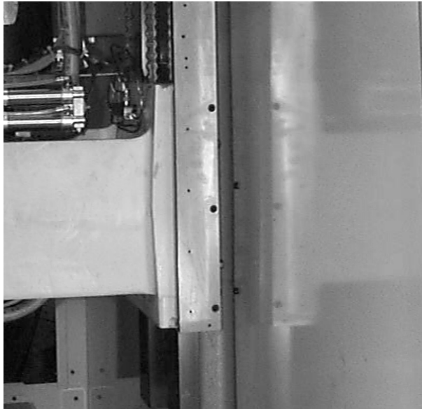
Figure 11-60 Attach Z Axis Mounting Plate to Side of Head Assembly
