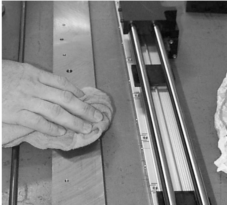
Figure 11-63 Thoroughly Clean Z Axis Mounting Plate
