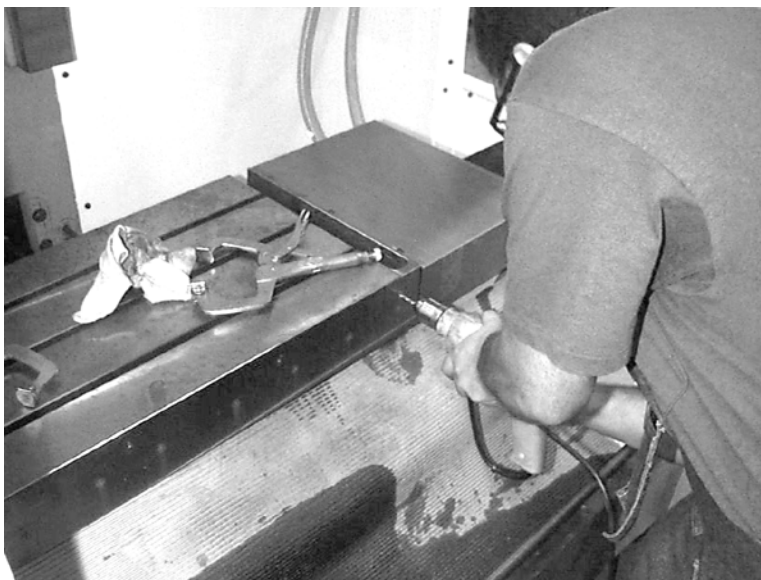
Figure 11-9 Counter Sink Holes
