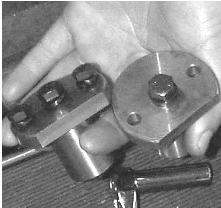
Figure 11-44 Insert Screws and Washers into Y Axis Scale Mounts
