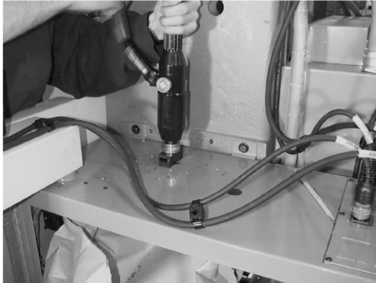
Figure 11-95 Create Opening for Fourth Axis Ribbon Cable
