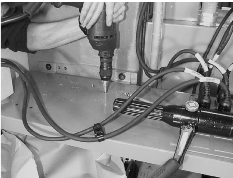
Figure 11-94 Open Holes with Step Drill
