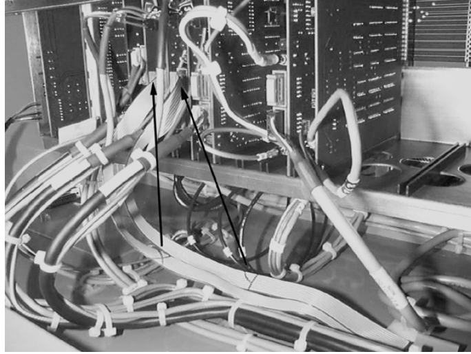
Figure 11-87 Secure Cable to Bottom of Cabinet
