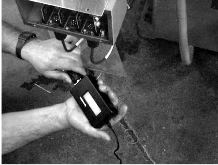
Figure 11-103 Plug Pin Connector Into Scale Test Box
