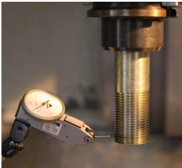
TEST SCREW IN SETUP WITH DIAL INDICATOR
