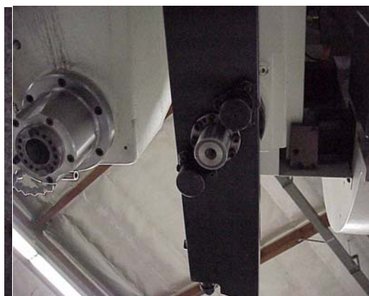
Figure 7-25: Insert and Tighten Installation Tool
