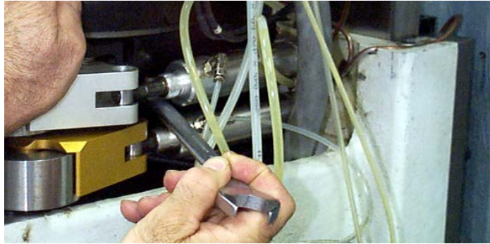
Figure 10-8: Remove Spindle Motor Bolt
