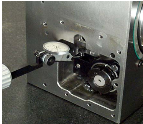
Figure 8-7: Zero Indicator on Worm Pivot Plate
