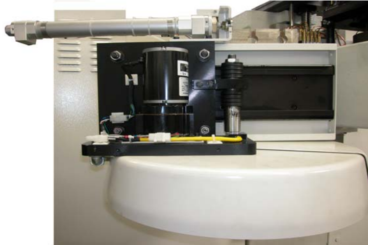
Figure 7-2: Move ATC Slide Toward Spindle
