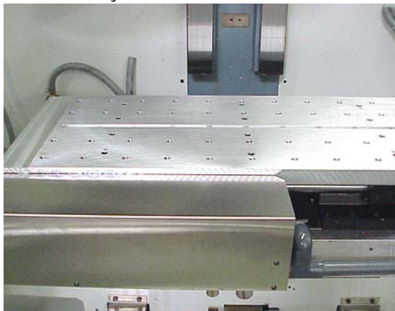
Figure 9-3 Remove Pallet Arm Safety Cover
