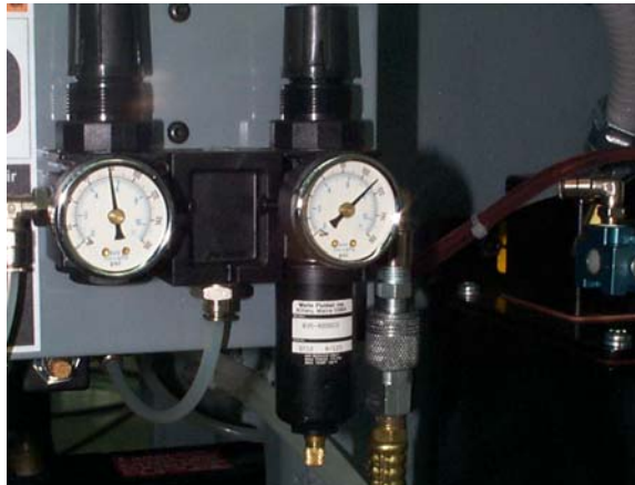
Figure 10-15: Dual Air Regulator Set at 80 psi and 120 psi
