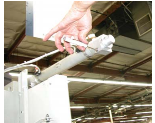
Figure 7-5: Loosen Hex Bolts / Move Slide to Spindle Until Engaged
