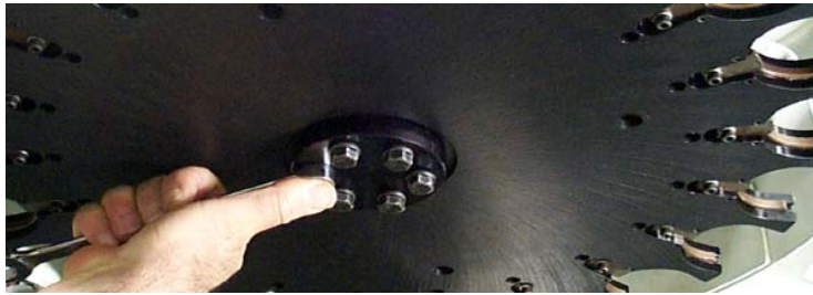
Figure 7-8: Loosen Hex Bolts on Under Side of Tool Carrier
