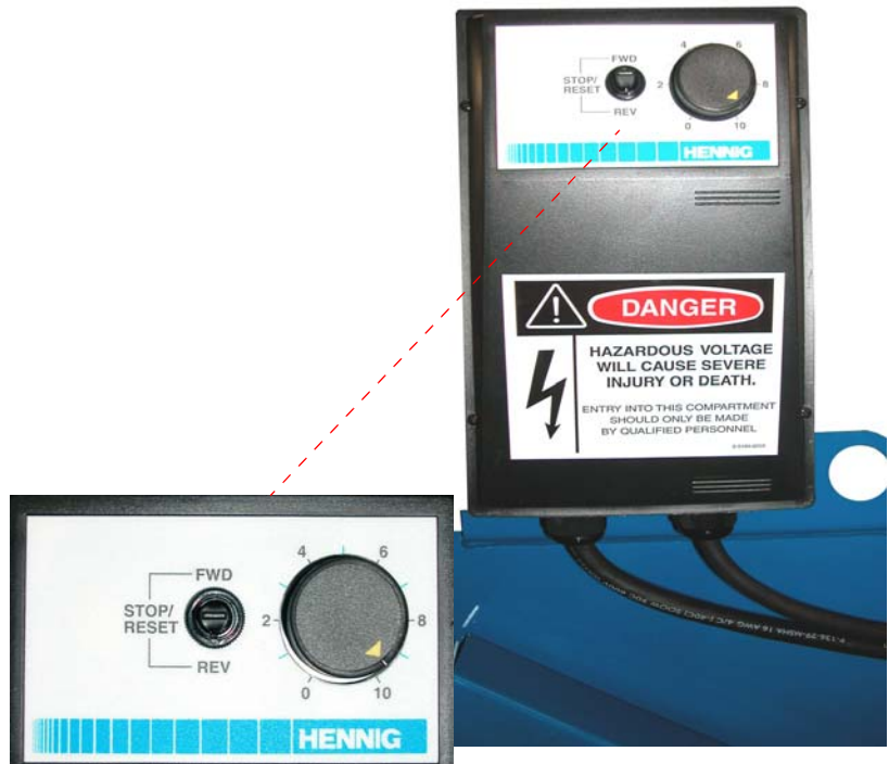
Figure 3-18: Control Operating Positions
