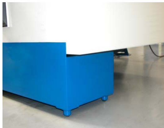
Figure 3-16: Place Sheet Metal Coolant Tank Slightly in Front of Machine Sheet Metal
