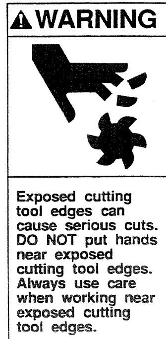
SAFETY LABEL NO. 5 EXPOSED CUTTING TOOLS SAFETY LABEL. LOCATED AS SHOWN IN THE ILLUSTRATION TITLED SAFETY LABEL LOCATIONS.
