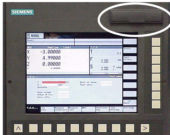
Figure 17 The PC card is inserted into the card slot of the operator panel for the HMI firmware installation.
