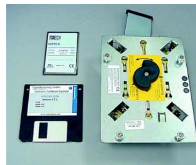
Figure 22 The files for performing the MMC103 software update are stored on a PC card and Utilities disk. The pre-imaged hard drive replaces the existing one in the MMC103 module.
